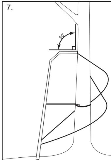
7. Cross Installation Straps behind tree. Attach to the top rung of the bottom ladder section. Pull to tighten the straps against the tree.
