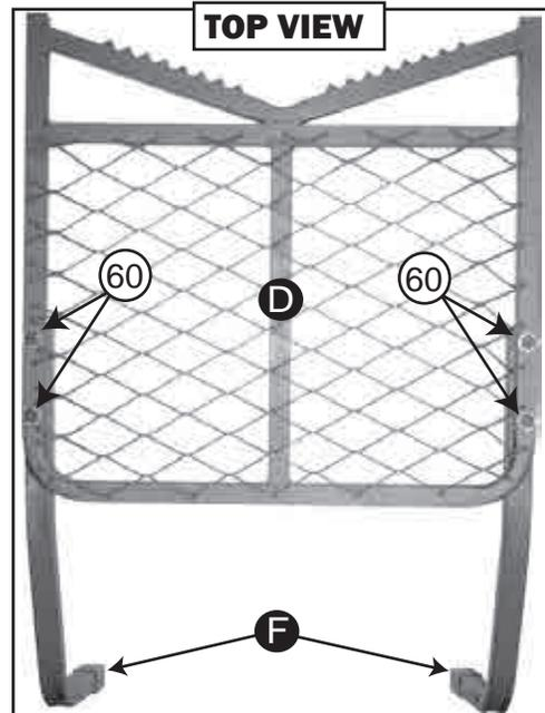
2. Attach Handle Rail **F** to the bottom of Seat Platform **D** using **2-M12x60mm bolts** on each side
