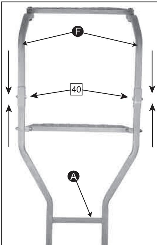
3. Insert sleeved end of Handle Rails **F** into Top Ladder Section **A**. Secure with 1-*M10x40mm bolt* on each side.
