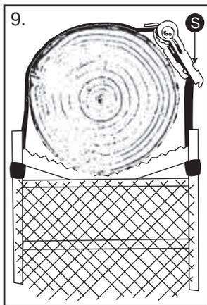
9. Wrap the strap of the ratchet around the back of the tree once and thread through the ratchet.
