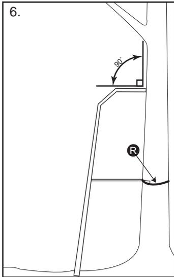
6. Tie one end of Tiedown Rope **R** to the inner part of Stabilizer Bar near the flanged end. Wrap the rope around the back of the tree once. Then tie the other end of the rope to the stabilizer bar.
