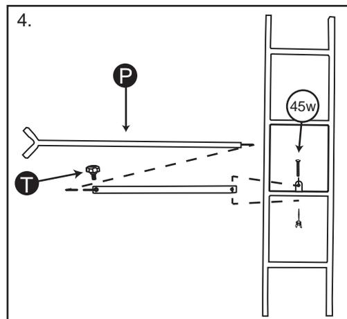
4. Slide the inner part of the Stabilizer Bar into the outer part. Attach Stabilizer Bar **P** to the second rung of the Middle Ladder Section with **1 - M12x45mm bolt and 1 wingnut**.
