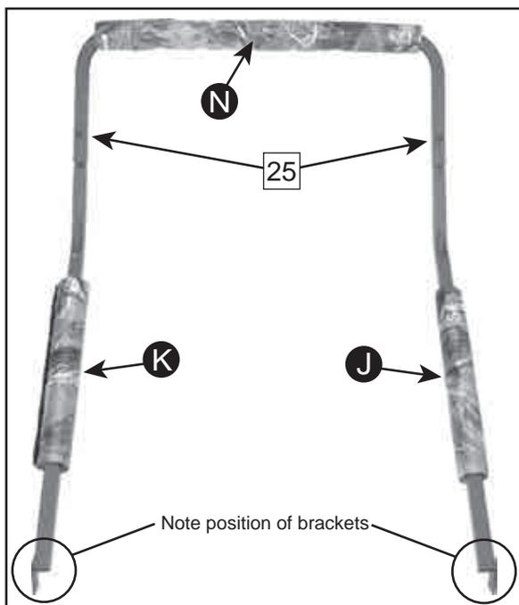
7. Insert each Shooting Rail Arm **J** and **K** into Shooting Rail **L**. Make sure that the welded tabs on each of the Shooting Rail Arms are on the outside and that the arm is angled up. Use **1-M10x25mm bolt** to secure in place.
