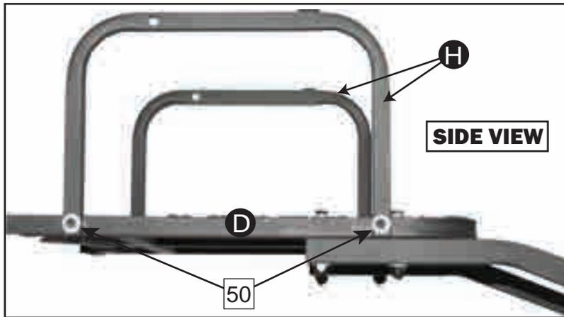
5. Attach each Arm Rest **H** to the sides of Seat Platform **D** using **2-M10x50mm bolt**.
