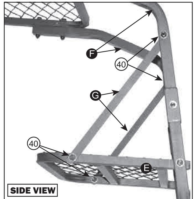
4. Attach one end of the Platform Support **G** to the **OUTSIDE** of Foot Platform **E** using 1-*M12x40mm bolt* for each side. Attach the other end of Platform Support **G** to the **INSIDE** of Handle Rail **F** using 1-*M12x40mm bolt* on each side.
