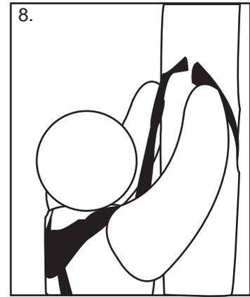
8. After the ladder stand has been secured to the tree with the installation straps, and the stabilizer bar has been securely attached to the tree, continue to have two people hold the ladder, climb cautiously up to the platform. Once you reach the top, **IMMEDIATELY ATTACH YOUR SAFETY HARNESS TO THE TREE.** Keep the tether strap above your head.
