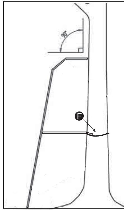
7. Slide the inner part of the Stabilizer Bar into the outer part. Attach Stabilizer Bar **D** to the top rung of the Theft Deterrent Ladder Section with **1 - M12x45w bolt and 1 wingnut**.
