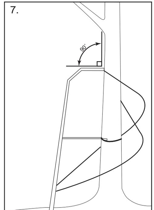
5. Move base of ladder toward or away from tree slightly in order to make Platform as parallel to the ground as possible.
