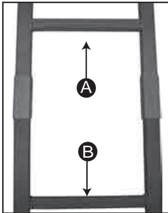
6. Insert Ladder Section **B** into the sleeved end of Top Ladder Section **A**.
