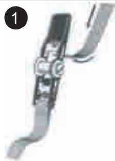
1. Open ratchet handle flat and insert end of strap through opening.
