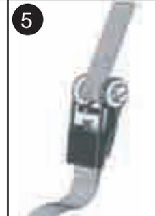
5. After strap is tight, close handle to the locked position
