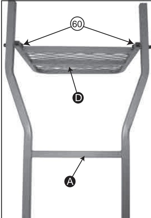
1. Attach Foot Platform **D** to the Top Ladder Section **A** using **1 - M12x60mm bolt** on each side.
