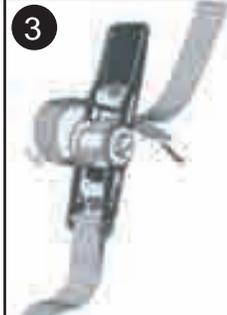
3. Insert tag end of strap back through slot in ratchet wheel.
