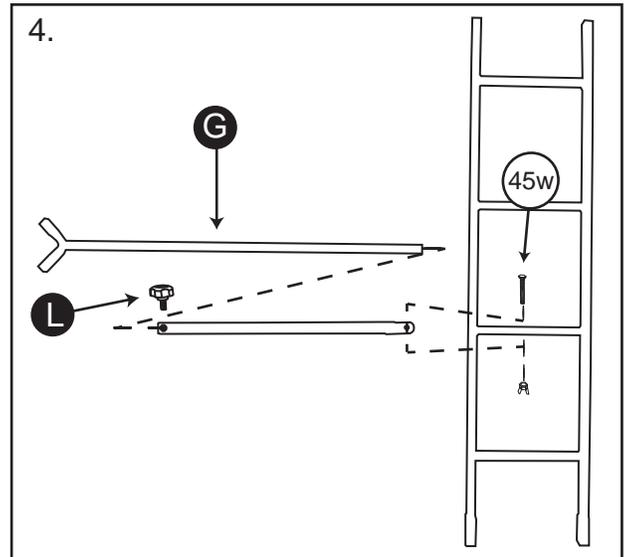
4. Slide the inner part of the Stabilizer Bar into the outer part. Attach Stabilizer Bar **G** to the second rung of the Middle Ladder Section with **1 - M12x45mm bolt and 1 wingnut**.
