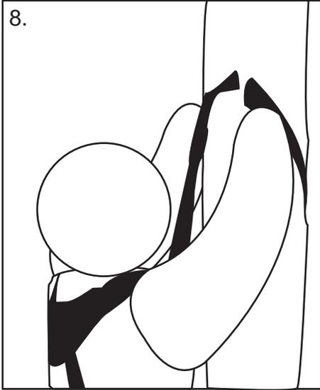
8. After the ladder stand has been secured to the tree with the installation straps, and the stabilizer bar has been securely attached to the tree, continue to have two people hold the ladder, climb cautiously up to the platform. Once you reach the top, **IMMEDIATELY ATTACH YOUR SAFETY HARNESS TO THE TREE.** Keep the tether strap above your head.
