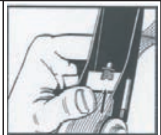
6 To release tension, push spring loaded retaining lock and simultaneously pull on strap.
