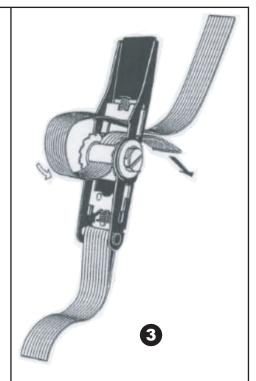
Insert tag end if strap back through slot in ratchet wheel.
