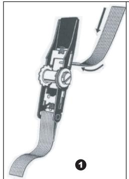
Open ratchet handle flat and insert end of strap through opening.
