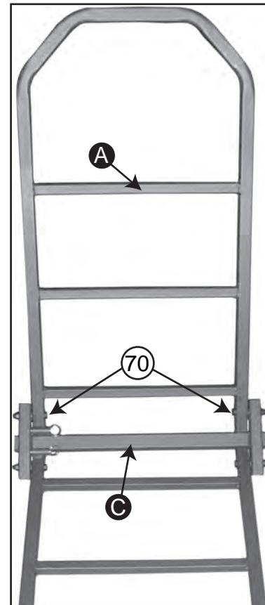
2. Attach Front Frame **A** to Axle Housing **C** to the rear most holes using **1-M12x70mm bolt** on each side. (See Closeup for proper installation order).
