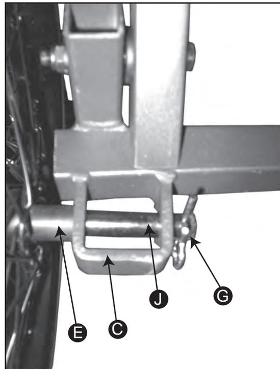
4. Insert Clevis Pin **J** through Axle Housing **C** .
