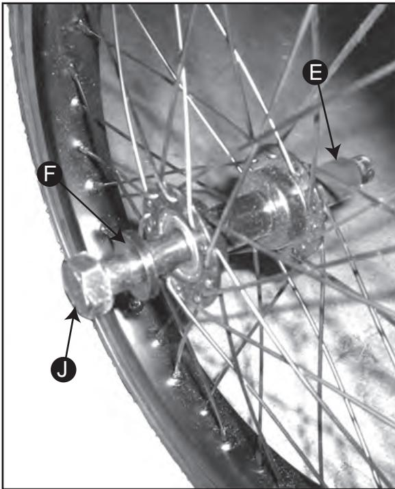
3. Slide Large Washer **F** onto Clevis Pin **J** .
