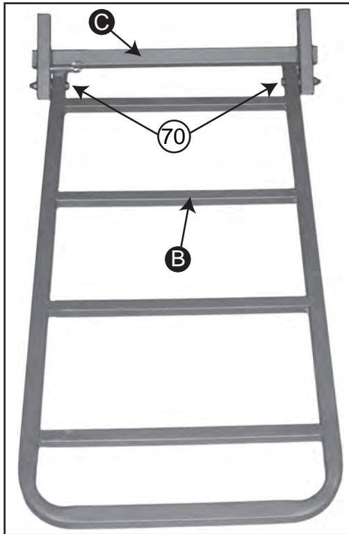
1. Attach Bottom Frame **B** to Axle Housing **C** to the front holes using **1-M12x70mm bolt** on each side. (See Closeup for proper installation order).
