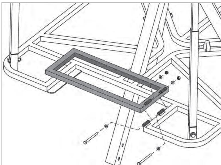
**Step 11:** Install **TRAP DOOR** to **PLATFORM** using (2) M6 x 70mm Bolts.
