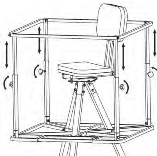
Loosen all four knobs to adjust Shooting Rail to a comfortable height.
