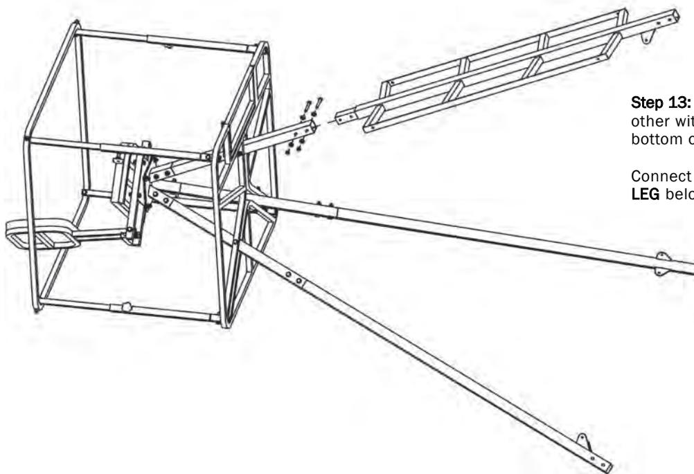
**Step 13:** Connect **MIDDLE LADDER LEG** to each other with **SHORT TRIPOD BRACE**, secure to tabs on bottom of **MIDDLE LEGS** using (2) M8 x 40mm bolt.
