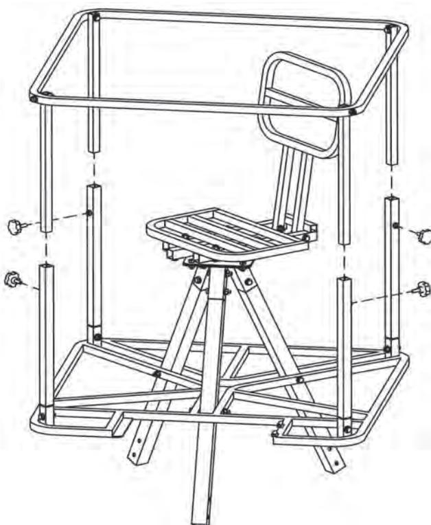
**Step 10:** Insert **SHOOTING RAIL** and **UPPER SHOOTING RAIL SUPPORTS** into **LOWER SHOOTING RAIL SUPPORTS**. Use (4) **ADJUSTMENT KNOBS** to connect both halves together.
