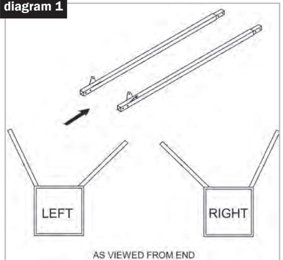
**Step 12:** Lay TRIPOD on its back as shown. Insert **RIGHT** and **LEFT MIDDLE LEGS** into **BOTTOM** of **UPPER LEGS** and secure with (4) M8 x 50mm bolts (2 bolts per leg).
