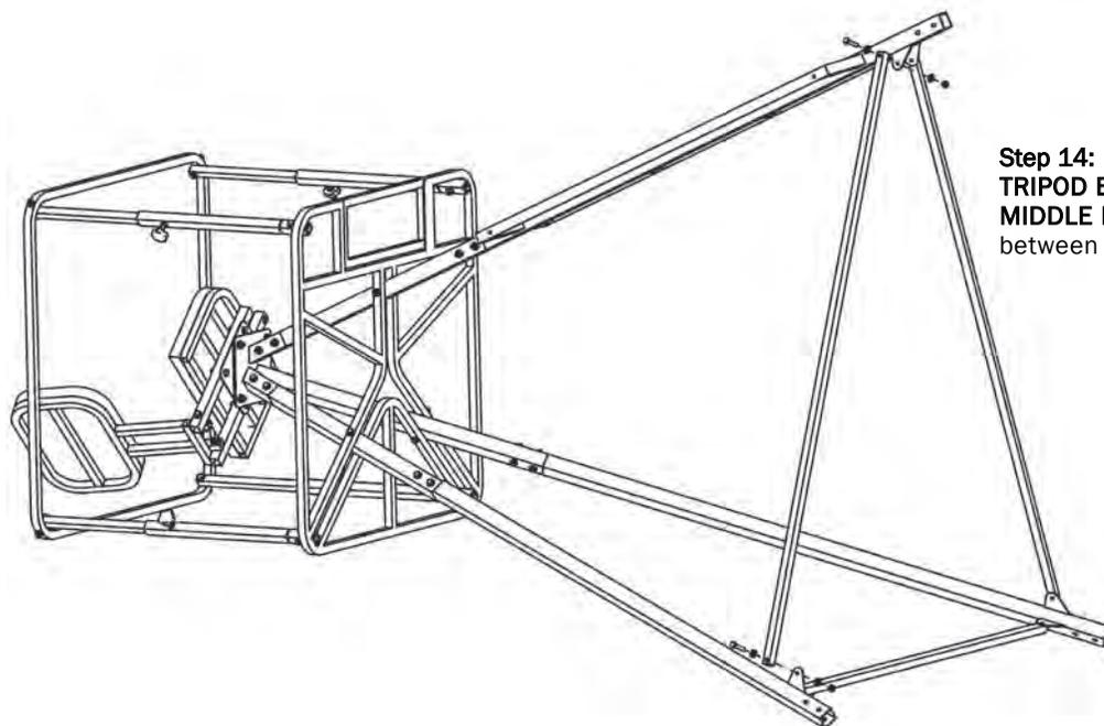
**Step 14:** Connect **ALL LEGS** by attaching (2) **LONG TRIPOD BRACES** from **MIDDLE LADDER LEG** back to **MIDDLE LEGS** and connect **SHORT TRIPOD BRACE** between **MIDDLE LEGS** using (6) M8 x 40mm bolts.
