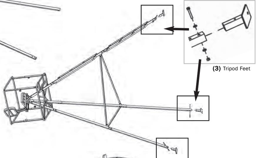
**Step 16:** Insert **TRIPOD FEET** into **BOTTOM LEGS** and secure using (3) M8 x 50 mm bolts.
