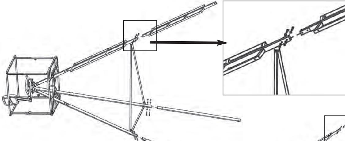
**Step 15:** Insert **BOTTOM LEGS** into **BOTTOM** of **MIDDLE LEG SECTIONS** and **BOTTOM LEG** into **BOTTOM** of **MIDDLE LEG** using (6) M8 x 50mm bolts to secure them all.
