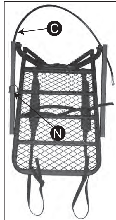
10. Insert one end of Cable C into Foot Platform Rail. Insert 1 - M8 Quickclip N into the rail and through the eyelet on the cable.
