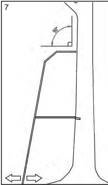
7. Move base of ladder toward or away from tree slightly in order to make Platform as parallel to the ground as possible.
