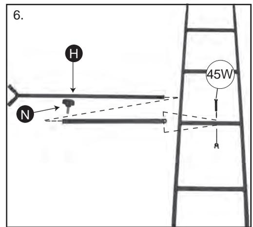
6. Slide the inner part of the Stabilizer Bar into the outer part. Attach Stabilizer Bar **H** to the second rung of the Middle Ladder Section with **1 - 12x45mm bolt and 1 wingnut**.
