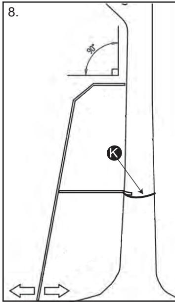
8. Tie one end of Tiedown Rope **K** to the inner part of Stabilizer Bar near the flanged end. Wrap the rope around the back of the tree once. Then tie the other end of the rope to the stabilizer bar.
