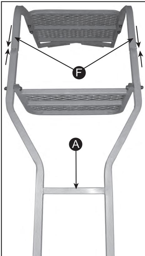
3. Slide the Top Ladder Section **A** into Handle Rails **F**.
