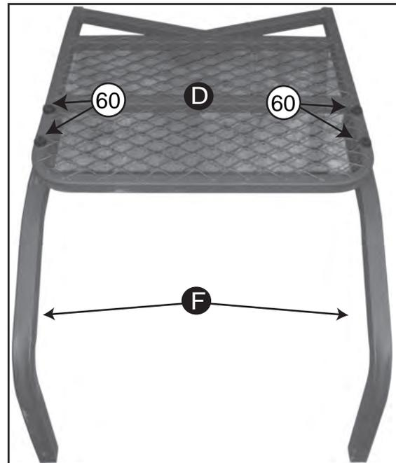
2. Attach each Handle Rail **F** to Seat Platform **D** using **2-M12x60mm bolts** on each side.
