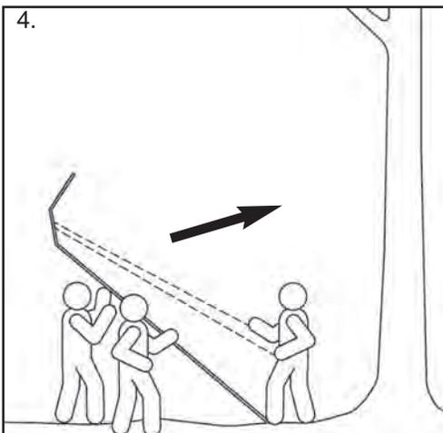
4. One person will stand at the base of ladder with his/her foot on bottom rung while holding installation straps. This will prevent tree stand from sliding. Two people will stand at opposite ends of tree stand, facing Platform and slowly walk tree stand upward using rungs of ladder.
