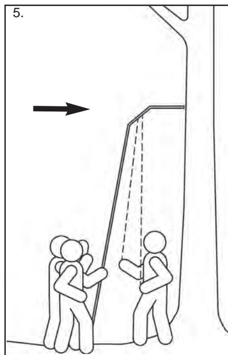
5. As tree stand is being raised, the person holding Installation Straps will pull toward themselves to take up slack. It will steady and ease the weight of stand on the other two people. Continue walking stand upward, until Tree Contact is resting against the tree.
