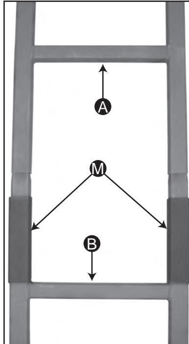
2. Insert Middle Ladder Section **B** into the Top Ladder Section **A**.
