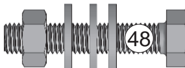
4 - M12x45mm (YELLOW) Bolt (3 Washers, 1 Lock-Nut)
