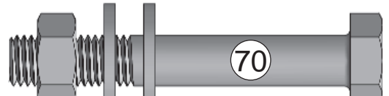
16 - M12x70mm (GREEN) Bolt (2 Washers, 1 Lock-Nut)
