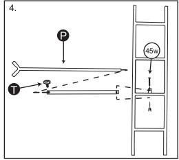
4. Slide the inner part of the Stabilizer Bar into the outer part. Attach Stabilizer Bar
