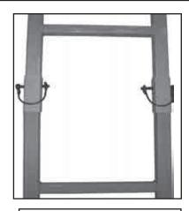
3. Close the quickclip to secure the ladder sections together.
