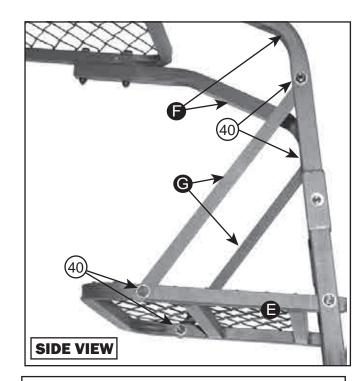
4. Attach one end of the Platform Support **6** to the **OUTSIDE** of Foot Platform **1** using **1-M12x40mm bolt** for each side. Attach the other end of Platform Support **6** to the **INSIDE** of Handle Rail **1** using **1-M12x40mm bolt** on each side.
