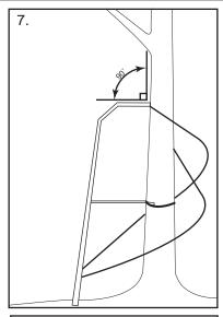
7. Cross Installation Straps behind tree. Attach to the top rung of the bottom ladder section. Pull to tighten the straps against
