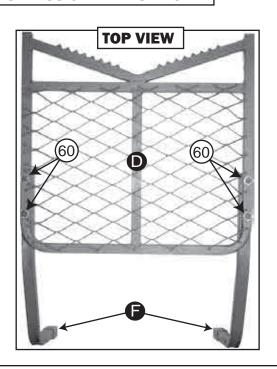
2. Attach Handle Rail **(F)** to the bottom of Seat Platform **(D)** using **2-M12x60mm bolts** on each side
