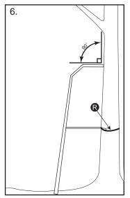
6. Tie one end of Tiedown Rope R to the inner part of Stabilizer Bar near the flanged end. Wrap the rope around the back of the tree once. Then tie the other end of the rope to the stabilizer bar.
