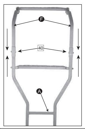
3. Insert sleeved end of Handle Rails **(F)** into Top Ladder Section **(A)**. Secure with *1-M10x40mm bolt* on each side.
