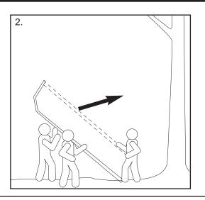
2. One person will stand at the base of ladder with his/her foot on bottom rung while holding installation straps. This will prevent tree stand from sliding. Two people will stand at opposite ends of tree stand, facing Platform and slowly walk tree stand upward using rungs of ladder.
