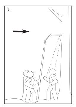
3. As tree stand is being raised, the person holding Installation Straps will pull toward themself to take up slack. It will steady and ease the weight of stand on the other two people. Continue walking stand upward, until Tree Contact is resting against the tree.
