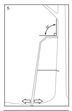
Move base of ladder toward or away from tree slightly in order to make Platform as parallel to the ground as possible.
