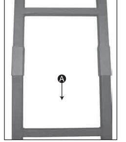
4. Insert Ladder Section (A) into the Original Middle Ladder Section .
