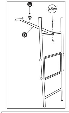
7. Slide the inner part of the Stabilizer Bar into the outer part. Attach Stabilizer Bar **()** to the top rung of the Theft Deterrent Ladder Section with **1** - *M12x45w bolt and 1 wingnut*.
