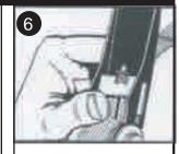
To release tension, push spring loaded retaining lock and simultaneously pull on strap.
