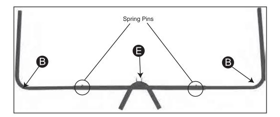
3. Slide each Rear Frame Corner **B** into Top Tree Brace **E**. The "U" part of the brace **MUST** be on top of the frame. **SEE CLOSEUP**
