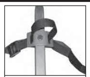
Pull strap over the top of the bracket, then through the other side of the bracket.
