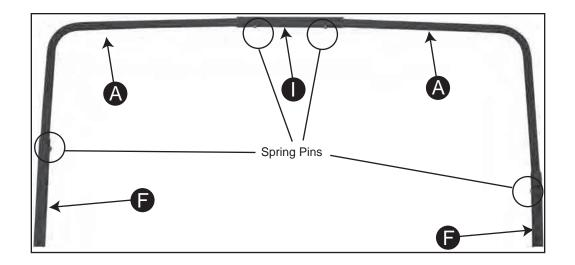
2. Slide each Side Brace onto the other end of Front Frame Corner
