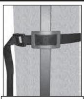
Wrap the Buckle Strap around the back of the tree and insert the strap through the buckle. Make sure that the strap is flat against tree with no slack.
