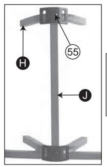
8. Attach remaining Bracket **(G)** to the top of Vertical Support **(J)** then attach to Bottom Tree Brace **(H)** with **1-M12x55mm bolt.**
