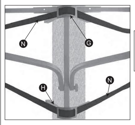
12. Raise the Roof Assembly to the tree using a safe hoist/lift system to 3 feet above the shooting rail of your treestand.
