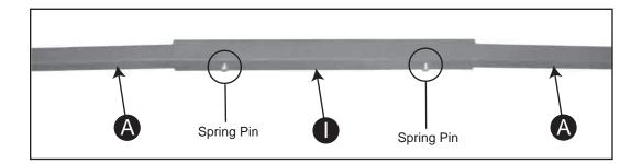
1. Slide Front Brace onto Front Frame Corner A .
