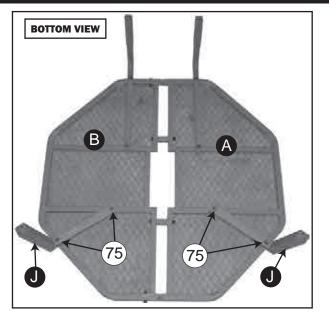
6. With the platform still upside down, Attach Rear Leg Brace to the rear of the platform using **2-M12x75mm Bolts** for each Rear Leg Brace.
