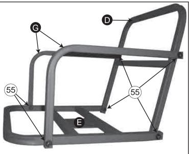
2. Attach Seat Back **D** to Seat Platform **E** using *1-M12x55mm Bolt* on each side.
