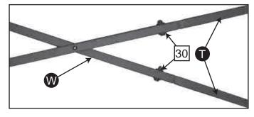
4. Insert the crimped end of Male Brace **1** into the end of Cross Brace **1** near the pivot point. Insert **1-M10x30mm Bolt** at each point. Do this for **ALL** remaining Cross Braces. Set aside for future use.
