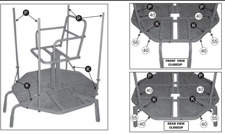
9. Attach Shooting Rail Support P the assembled platform using **1-M12x55mm Bolt** for each piece. (See Close-Up Photo for correct placement).
