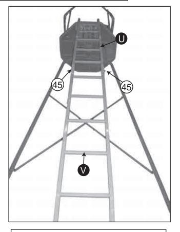
16. Insert Bottom Ladder Section **(V)** into Top Ladder Section **(U)**. The brackets on the Ladder Section **MUST** be facing towards the inside of the stand. Secure using **1-M12x45mm Bolt** on each side.
