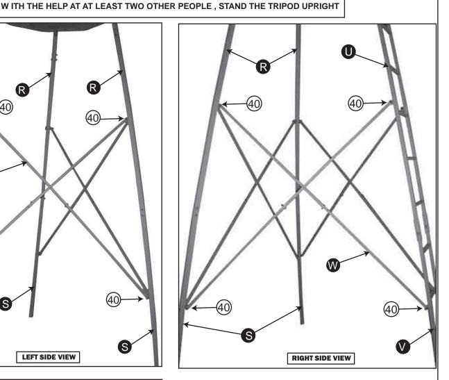
18. Attach the last Cross Brace W to Top Ladder Section U and Lower Leg S . Attach the same Cross Brace to Bottom Ladder Section **W** and Upper Leg **R** using **1-M12x40mm Bolt** at each point. Attach Braces to the OUTSIDE of the Brackets.
