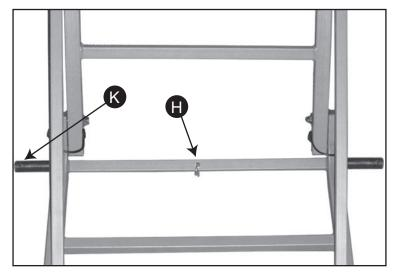
3. Insert Axle ( through Bottom Frame ). Line the holes up on the axle and the center of the bottom frame. Insert Large Cotter Pin ( to secure in place.
