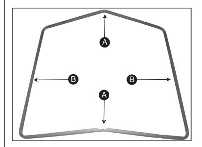
1. Insert each Roof Frame A into each Roof Frame Side B.
