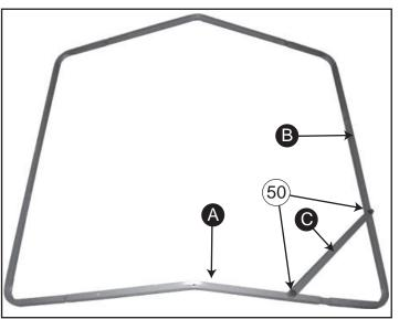
2. Attach Frame Brace **(C)** to the top of Roof Frame **(A)** and Roof Frame Side **(B)** using **1-M10x50mm Bolt** at each point.
