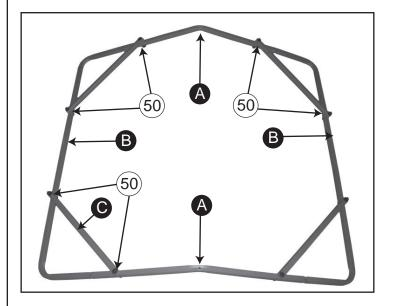
3. Attach the remaining Frame Braces to the top of Roof Frame and Roof Frame Sides using *1-M10x50mm bolt* at each point.
