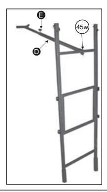
7. Slide the inner part of the Stabilizer Bar into the outer part. Attach Stabilizer Bar **(1)** to the top rung of the Theft Deterrent Ladder Section with 1 - M12x45w bolt and 1 wingnut.
