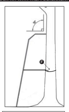
9. Tie one end of Tiedown Rope to the inner part of Stabilizer Bar near the flanged end. Wrap the rope around the back of the tree once. Then tie the other end of the rope to the stabilizer bar.
