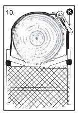
10. Cautiously climb to the top of the treestand. Wrap the strap of the ratchet around the back of the tree once and thread through the ratchet. (See Detailed Ratchet Instructions Below)
