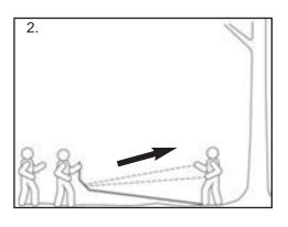
2. Position bottom of stand 4-5 feet from base of tree.
