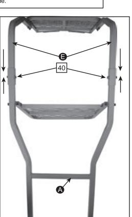
3. Slide the Top Ladder Section A into the Handle Rails . Secure with 2-M10x40mm
