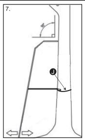
7. Tie one end of Tiedown Rope ① to the inner part of Stabilizer Bar near the flanged end. Wrap the rope around the back of the tree once. Then tie the other end of the rope to the stabilizer bar.
