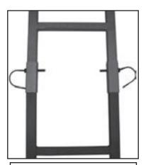
2. Insert **1 - Quickclip** through the hole on the sleeve, and through the ladder sections on each side of the ladder.
