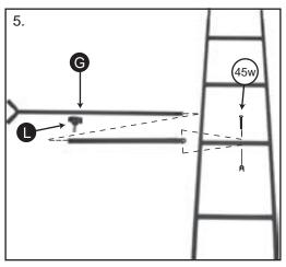
5. Slide the inner part of the Stabilizer Bar into the outer part. Attach Stabilizer Bar **(G)** to the second rung of the Middle Ladder Section with 1 - M12x45mm bolt and 1 wingnut.
