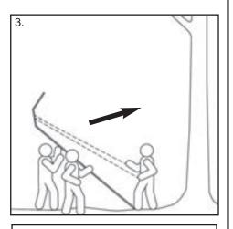
3. One person will stand at the base of ladder with his/her foot on bottom rung while holding installation straps. This will prevent tree stand from sliding. Two people will stand at opposite ends of tree stand, facing Platform and slowly walk tree stand upward using rungs of ladder.
