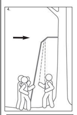
4. As tree stand is being raised, the person holding Installation Straps will pull toward themself to take up slack. It will steady and ease the weight of stand on the other two people. Continue walking stand upward, until Tree Contact is resting against the tree.
