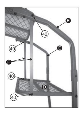
4. Attach one end of the Platform Support to Foot Platform using *1-M12x40mm bolt* for each side. Attach the other end of Platform Support to the inside of Handle Rail using *1-M12x40mm bolt* on each side.
