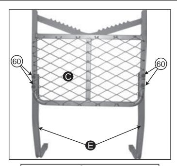
2. Attach Handle Rail **(a)** to the bottom of Seat Platform **(b)** using **2-M12x60mm bolts** on each side.
