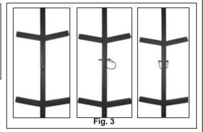
3. Thread the buckle strap through one end of the bracket, over the top of the bracket, then through the other side of the bracket. Pull the strap all the way through so the buckle end is against the bracket. The straps will be attached to the bracket and hang freely until the Stick Ladder is ready to be secured to the tree.
