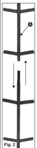
2. With the help of at least **TWO** other people, lower your assembled stick ladder to the ground. Lay your current stick ladder on the ground and insert the extension between the middle ladder sections of your stick ladder.
