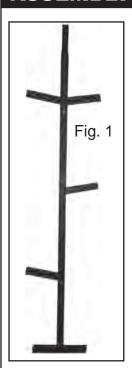
1. Lay Bottom Section **©** on the ground with the first step on the left hand side. (Fig. 1).
