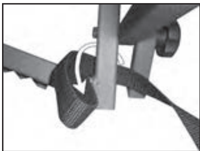
1. Place looped end of strap under platform.
