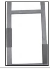
3. Slide the Sleeves over the joint where ladder sections are connected.
