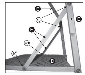
5. Attach one end of the Platform Support **F** to Foot Platform **D** using **1** - **M12x40mm bolt** for each side. Attach the other end of Platform Support **F** to the inside of Handle Rail **E** using **1** - **M12x40mm bolt** on each side.
