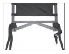
2. Attach Ratchet 🔘 to the outermost corners of the Handle Rail just behind the Installation Ropes. (See Ratchet Instructions.)
