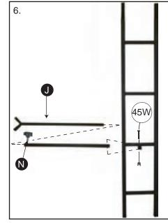
6. Slide the inner part of the Stabilizer Bar into the outer part. Attach Stabilizer Bar ① to the **bracket** on the **second rung from the bottom of the middle ladder section** with **1 - M12x45W bolt and 1 wingnut**.
