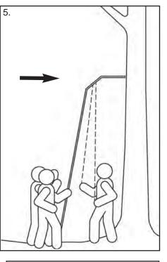
5. As tree stand is being raised, the person holding the installation straps will pull toward themself to take up slack. It will steady and ease the weight of stand on the other two people. Continue walking stand upward, until Tree Contact is resting against the tree.
