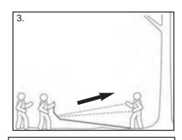
3. Position bottom of stand 4-5 feet from base of tree.
