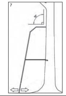
7. Move base of ladder toward or away from tree slightly in order to make Platform as parallel to the ground as possible.
