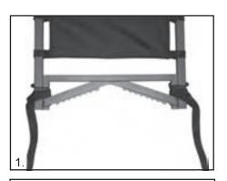
1. Attach Installation Cross Straps **(x)** to the rear of Seat Platform as shown. **(See Installation Strap Instructions)**
