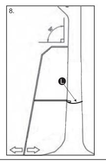
8. Tie one end of Tiedown Rope () to the inner part of Stabilizer Bar near the flanged end. Wrap the rope around the back of the tree once. Then tie the other end of the rope to the stabilizer bar.
