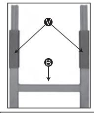
1. Slide Sleeves **V** over the crimps of Middle Ladder Section **B** .
