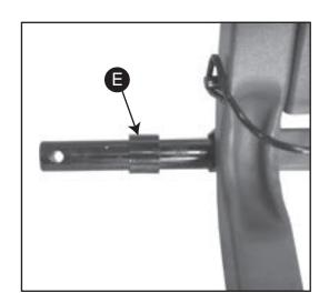
4. Slide Bushing **(a)** over each side of Axle **(b)**.
