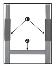
4. Slide Sleeves **F** over the crimps of Ladder Section **A**.
