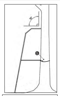
11. Tie one end of Tiedown Rope **(G)** to the inner part of Stabilizer Bar near the flanged end. Wrap the rope around the back of the tree once. Then tie the other end of the rope to the stabilizer bar.
