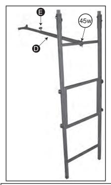
9. Slide the inner part of the Stabilizer Bar into the outer part. Attach Stabilizer Bar **1** to the top rung of the Theft Deterrent Ladder Section with 1 - M12x45w bolt and 1 wingnut.
