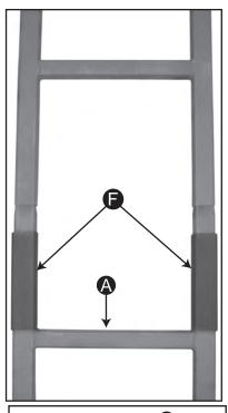
5. Insert Ladder Section A into the Original Middle Ladder Section .
