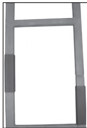
18. Slide the Sleeves over the joint where ladder sections are connected.
