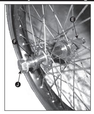
3. Slide Large Washer onto Clevis Pin .
