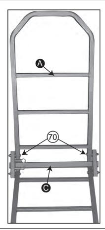
2. Attach Front Frame A to Axle Housing to the rear most holes using 1-M12x70mm bolt on each side. (See Closeup for proper installation order).
