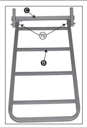
1. Attach Bottom Frame **(B)** to Axle Housing **(C)** to the front holes using *1-M12x70mm bolt* on each side. **(See Closeup for proper installation order).**
