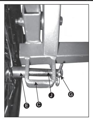
4. Insert Clevis Pin through Axle Housing Insert Cotter Pin through hole on Clevis Pin.
