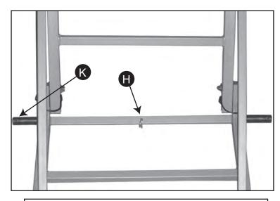
3. Insert Axle (K) through Bottom Frame (B). Line the holes up on the axle and the center of the bottom frame. Insert Small Cotter Pin (F) to secure in place.
