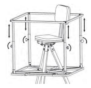
Loosen all four knobs to adjust Shooting Rail to a comfortable height.
