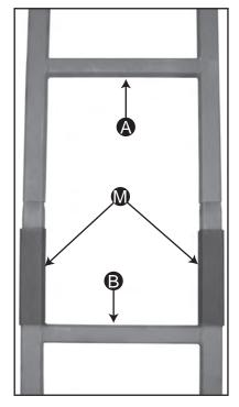
2. Insert Middle Ladder Section **B** into the Top Ladder Section **A**.
