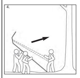
4. One person will stand at the base of ladder with his/her foot on bottom rung while holding installation straps. This will prevent tree stand from sliding. Two people will stand at opposite ends of tree stand, facing Platform and slowly walk tree stand upward using rungs of ladder.
