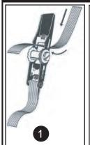
Open ratchet handle flat and insert end of strap through opening.
