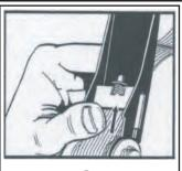
To release tension, push spring loaded retaining lock and simultaneously pull on strap.
