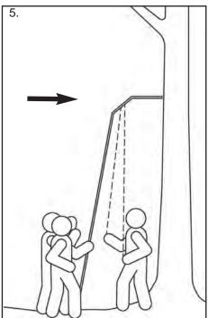
5. As tree stand is being raised, the person holding Installation Straps will pull toward themself to take up slack. It will steady and ease the weight of stand on the other two people. Continue walking stand upward, until Tree Contact is resting against the tree.
