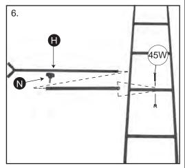
6. Slide the inner part of the Stabilizer Bar into the outer part. Attach Stabilizer Bar (1) to the second rung of the Middle Ladder Section with 1 - 12x45mm bolt and 1 wingnut.
