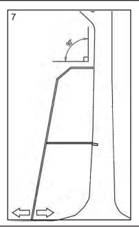
Move base of ladder toward or away from tree slightly in order to make Platform as parallel to the ground as possible.
