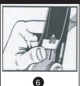
To release tension, push spring loaded retaining lock and simultaneously pull on strap.
