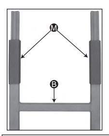
1. Slide Sleeves **M** over the crimps of Middle Ladder Section **B**.
