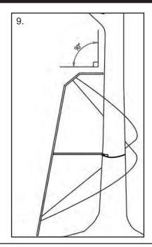
9. Cross Installation Straps behind tree. Attach to the bottom ladder section by following Installation Strap Instructions Steps 4-8.
