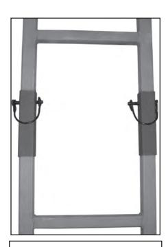
5. Close the quickclip to secure the ladder sections together.
