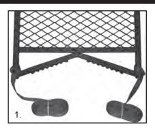
1. Attach Installation Cross Straps 1 to the rear of the seat platform by following Installation Strap Instructions.
