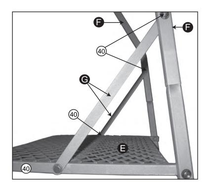
4. Attach one end of the Platform Support **G** to Foot Platform **E** using **1** - **M12x40mm bolt** for each side. Attach the other end of Platform Support **G** to the inside of Handle Rail **F** using **1** - **M12x40mm bolt** on each side.
