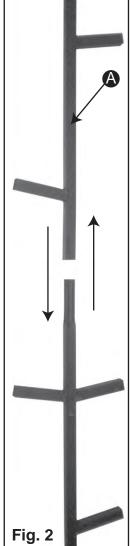
2. With the help of at least **TWO** other people, lower your assembled stick ladder to the ground. Lay your current stick ladder on the ground and insert the extension into the highest ladder section of your stick ladder that is not the top section. (See Fig. 2) Insert *1-Quickclip* into the new section at the insertion point. (See Fig. 3)
